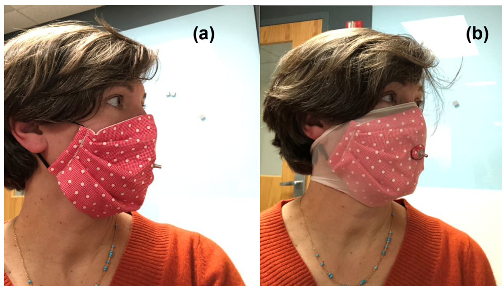
Figure 2. Facemask (Mask D) worn as designed (a) and with a nylon stocking layer (b) with tightly-sealed grommet positioned at the philtrum of the upper lip. The grommet is used to sample air from inside the mask during testing.
