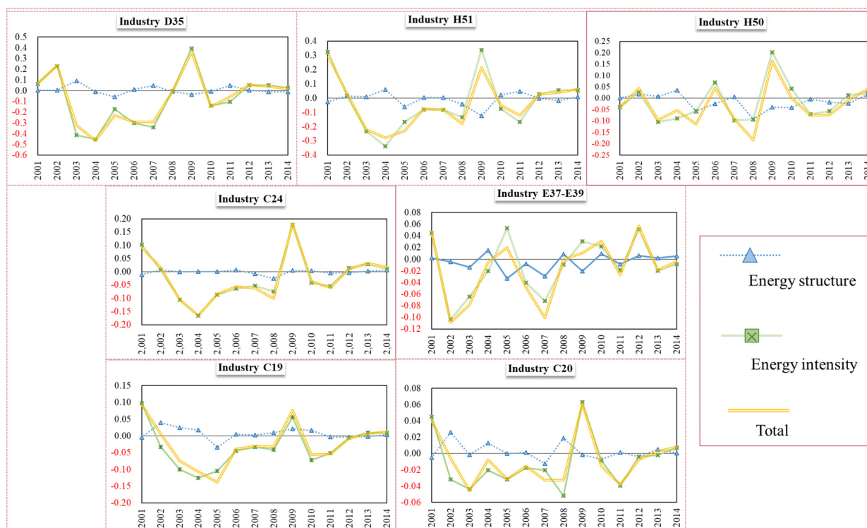
Fig. 7. Carbon intensity decomposition analysis of industries with large initial carbon intensity (initial carbon intensity \geq 0.5\text{tpt} ). 3.3.2 Carbon intensity decomposition analysis of remaining industries.
